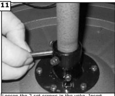
Loosen the 2 set screws in the yoke. Insert downrod into yoke, aligning large hole in the downrod with the large hole in the yoke. Insert cross pin though yoke and downrod.
